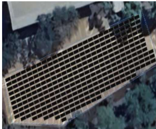
Figure 27 - Carport P2 - 172.15 kWp (Assumes New Structure)
