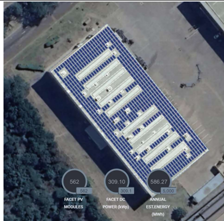
Figure 13 - Roof A5 - 309.1 kWp
