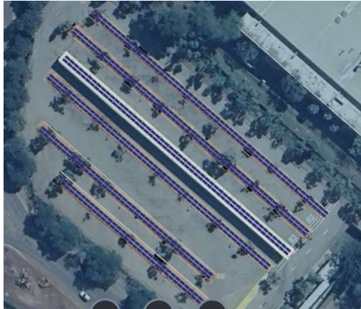
Figure 29 - Taxi Rank - 300.8 kWp
